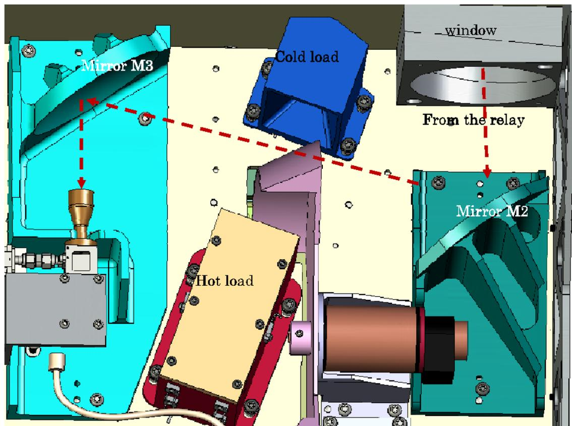
Figure 20. Optical layout within the WVR encasing, showing the loads, the chopper vane and the input feed to the mixer.
