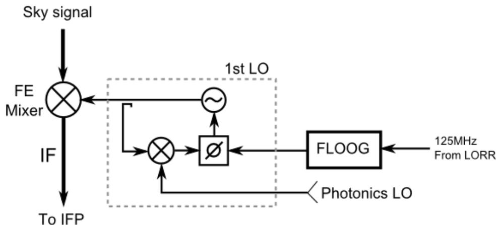
Figure 78. Block diagram of the WCA Fringe Tracking and Down-converting system.
