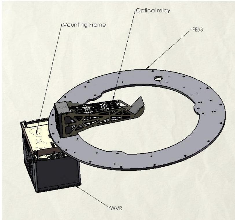
Figure 19. Offset optics used to collect the sky emission along the optical axis of the antenna into the WVR.
