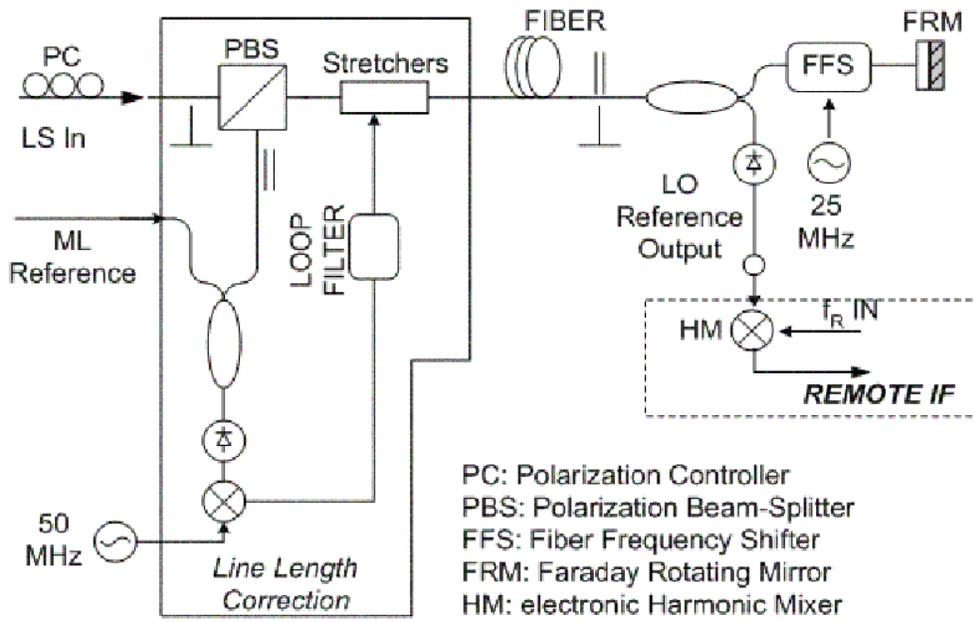
Figure 77. Block diagram of the Line Length Corrector system for ALMA.
