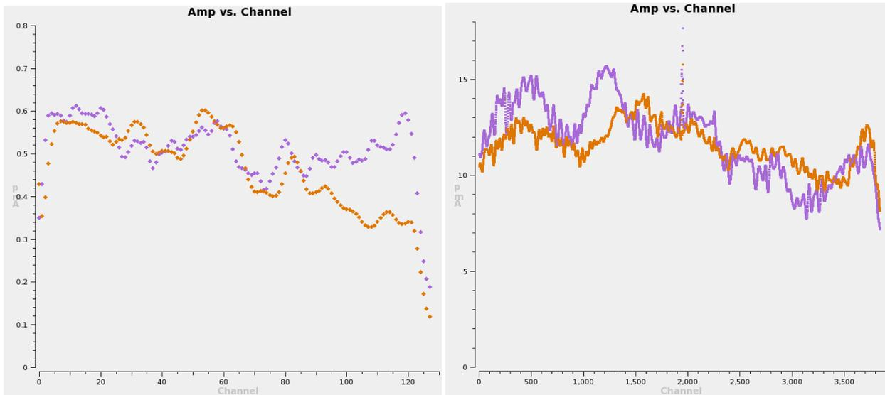
Figure 27. Comparison of TDM (left) and FDM (right) showing the dropoff in total power at the edges in the two modes. Colours represent the two polarisations from an example antenna. The 2.0 GHz bandwidth output from the correlator in TDM mode shows the drop in power in the upper and lower ~4 channels due to the anti-aliasing filter. In FDM, only the central 1.875 GHz is output from the correlator, and the drop in power at the edges of this bandwidth is negligible.
