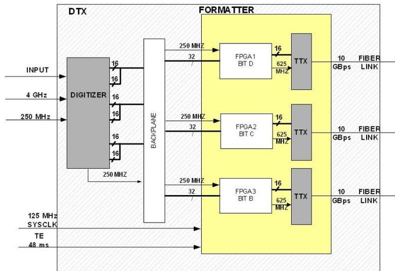
Figure 73. The DTX and DRX Signal Digitization and Transmission system.
