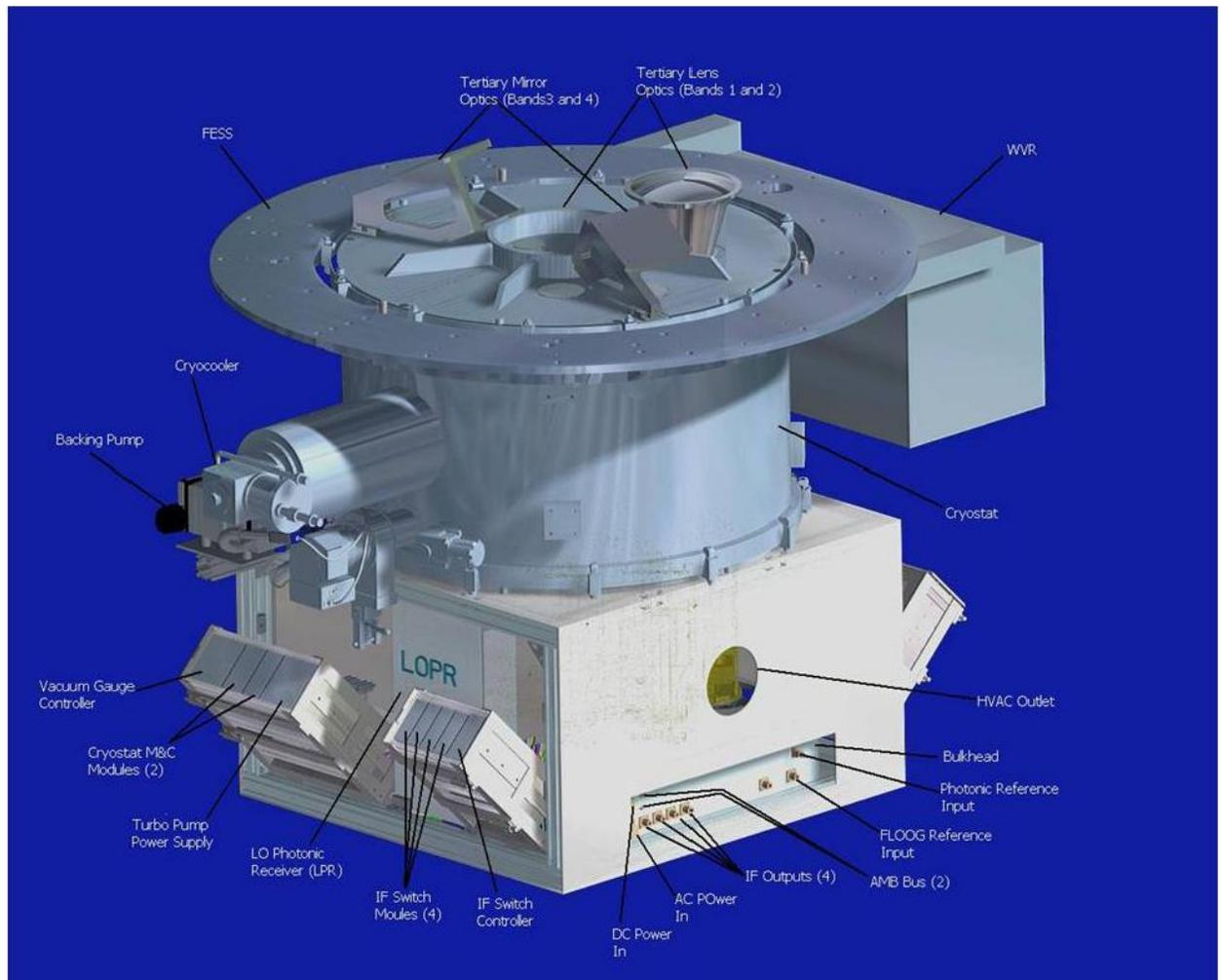
*Figure 67: Side view of ALMA frontend showing cryostat assembly, with room temperature unit below.*
