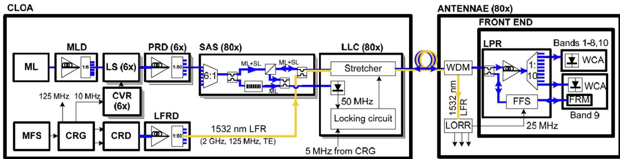
Figure 74. LO block diagram, showing the Central LO (CLOA) and the LO section in the WCA in each frontend. For description of acronyms, see text.
