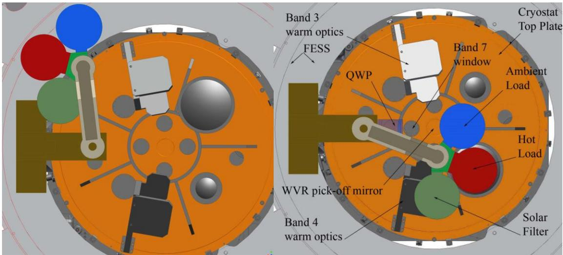
*Figure 22.* Top view of an ALMA front end showing the robotic arm of the ACD retracted during normal observations or on top of one of the front-end inserts for calibration. The current design has been improved by placing all the loads in a wheel.
