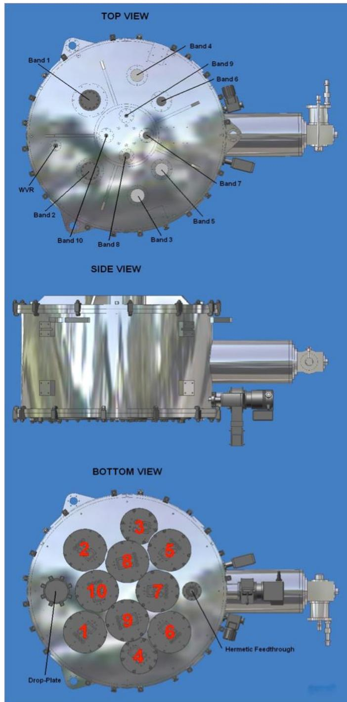
Figure 69. Views of cryostat assembly, showing different windows (top) and the portholes for the WCAs for each band (lower view).
