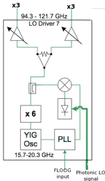
Figure 71. Block diagram of LO1 generation in a WCA - in this case Band 7 (diagrams for the other bands are shown in the description of the individual bands). Note that an additional multiplier (in this case, x3) is used to generate the LO1 frequency, at 282.9 – 365.1GHz.
