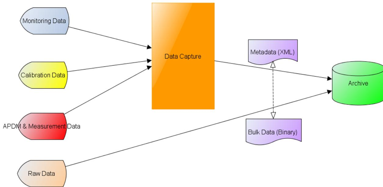
Figure 58. Data flow components.
