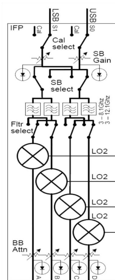
Figure 72. Block diagram of IF Processor.
