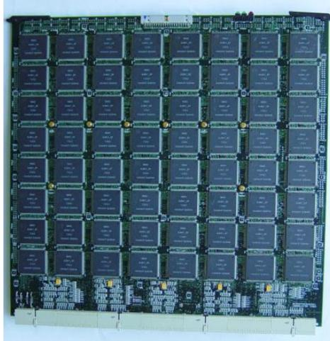
Figure 24. Correlator board, with the 8x8 array of custom correlator chips, each with 4k lags. There are 128 such boards per correlator quadrant adding up to a grand total of 32768 chips.
