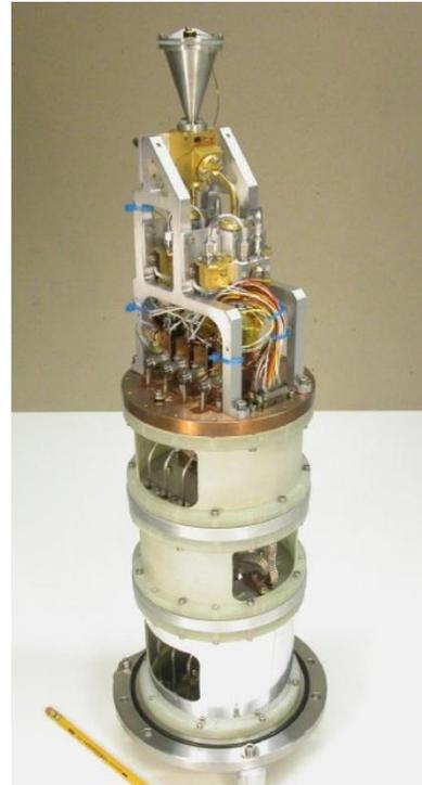
Figure 4. Block diagram of the Band 3 receiver (left) including CCA (upper) and WCA (lower). Right image shows a Band 3 CCA. Note the single feedhorn which feeds the OMT, splitting the two polarization signals for the 2SB mixers. The Band 3 cartridges are constructed in Canada at NRC-HIA, Victoria.
