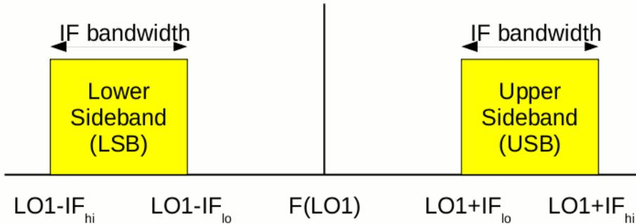
Figure 2. IF ranges for the two sidebands in a heterodyne receiver.
