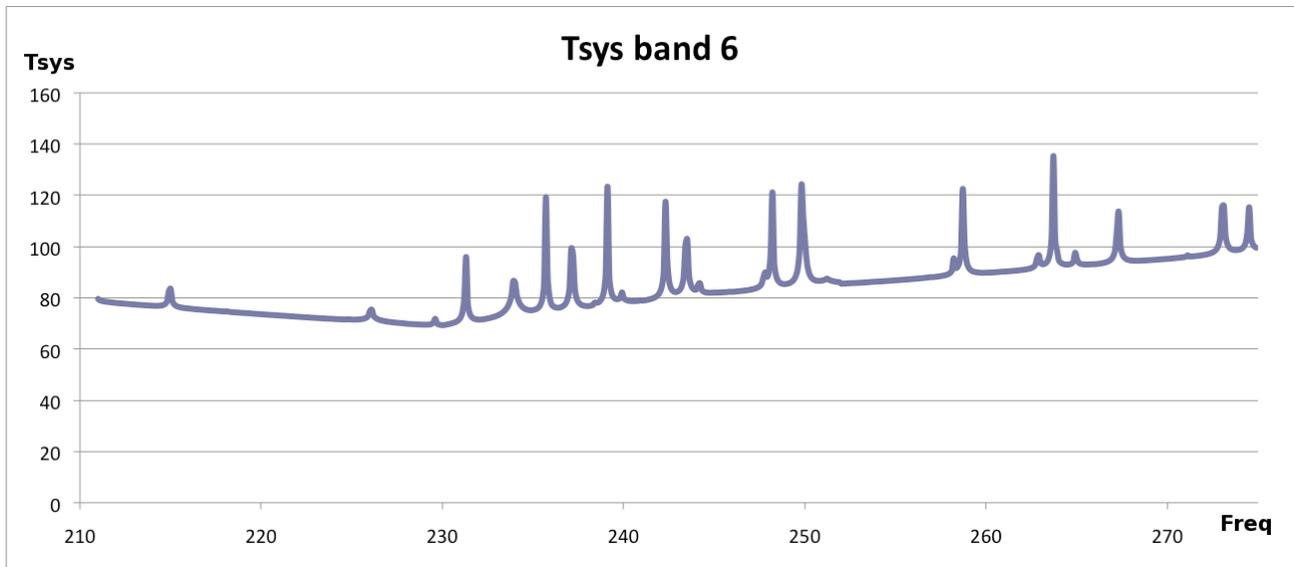
Figure 10. Typical  $T_{\text{sys}}^3$  at zenith for Band 6 with 1mm pwv, based on measured values of the receiver temperatures.
