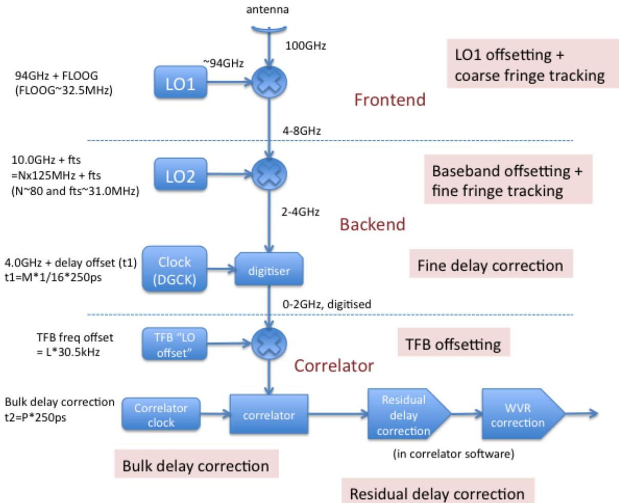
Figure 70. Summary of LO mixing scheme. Example frequencies are given for an observation at a
