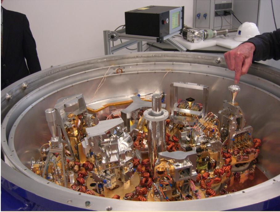
Figure 14: An open cryostat being shown off to guests at the ALMA Inauguration in March 2013. The demonstrator is pointing to the feedhorn of a Band 3 receiver. During Cycle 2, all antennas will be equipped with receivers covering Bands 3, 4, 6, 7, 8 and 9. (Credit: J. Hesser)
