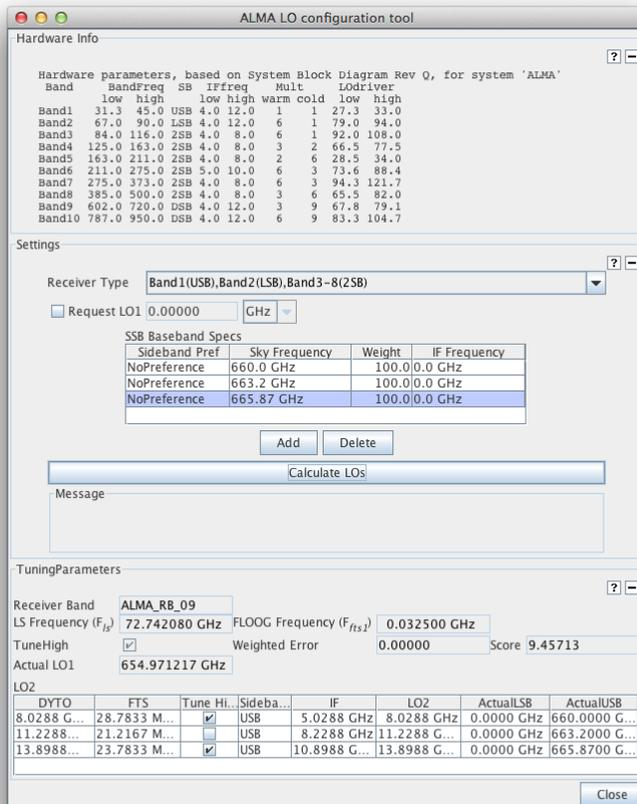
Figure 7.6: The LO Configuration Tool. Three Band-9 basebands have been requested with the tuning results shown at the bottom.
