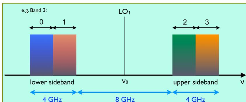
Figure 33: A graphical view of basebands and sidebands. Basebands may be tuned to overlap if the user wishes, or may be located so as to maximize the total bandwidth (as shown). Each baseband may be further subdivided into as many as 8 spectral windows. Up to four spectral windows per baseband are available.
