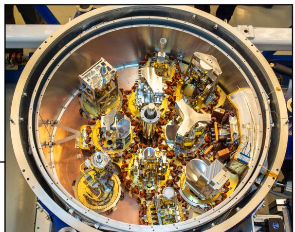
Figure 35: An open cryostat fitted with receivers covering Bands 1 through 10, including the prototype Band 2 cartridge. When fully populated, ALMA will have complete coverage available from the ground from 35 GHz to 950 GHz. (Credit: ALMA (ESO/NAOJ/NRAO); Sergio Otarola)
