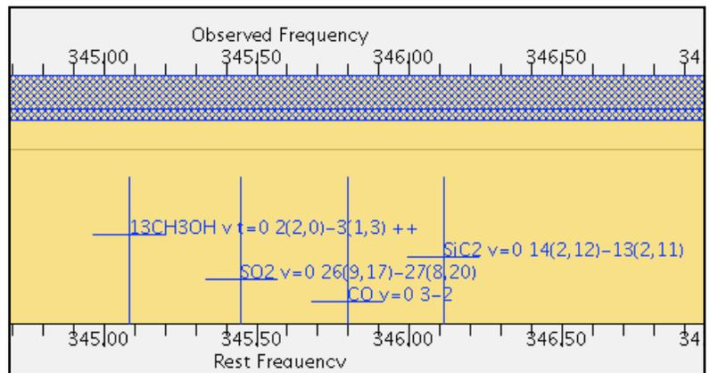
Figure 38: Four spectral windows were set up to observe these four lines simultaneously in one baseband using the OT. The windows are each 234 MHz wide (with 0.43 km/s channels), and are centered at 345.80, 345.45, 346.11 and 345.09 GHz. The spectral windows must fit within the 2 GHz wide baseband.
