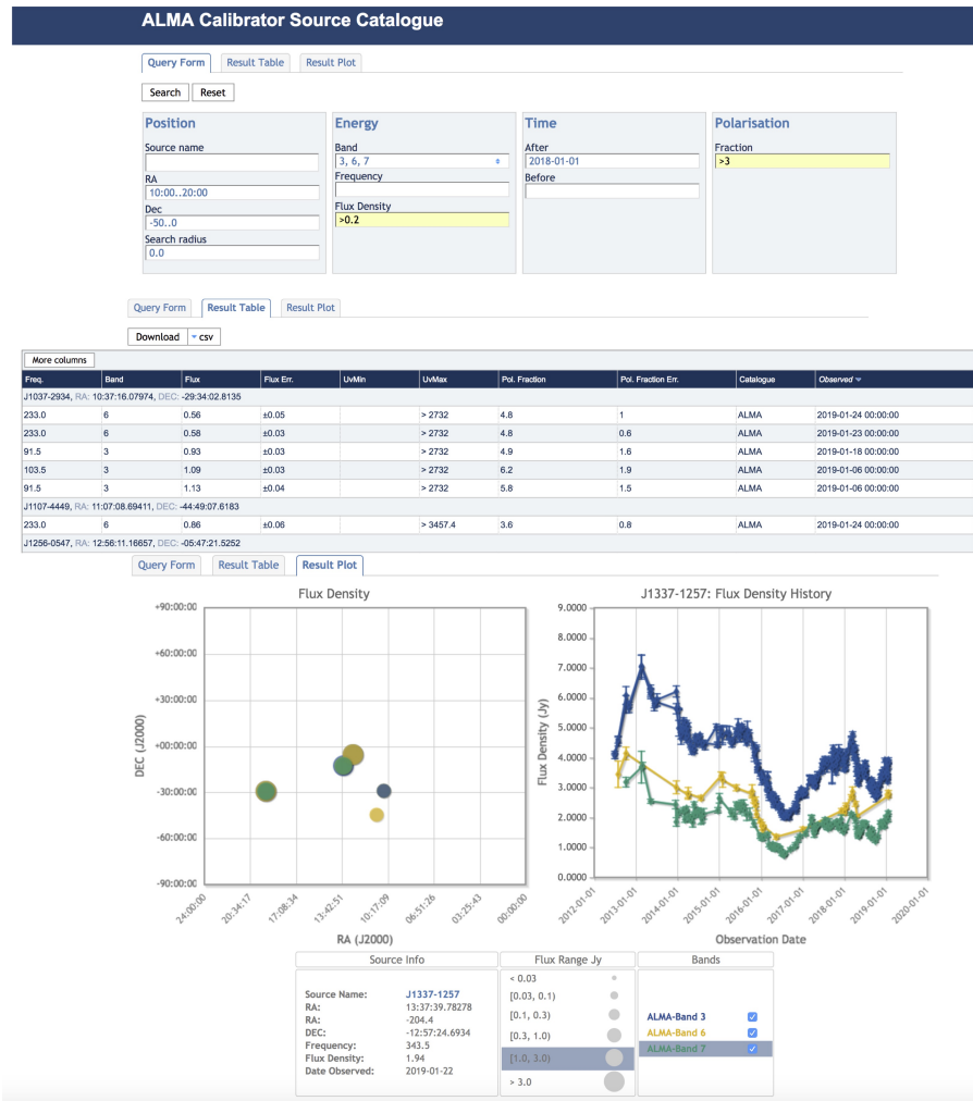
Figure 13.2: Example of a search for polarized calibrators in an RA/Dec range with recent measurements and a flux density limit for a set of ALMA bands
