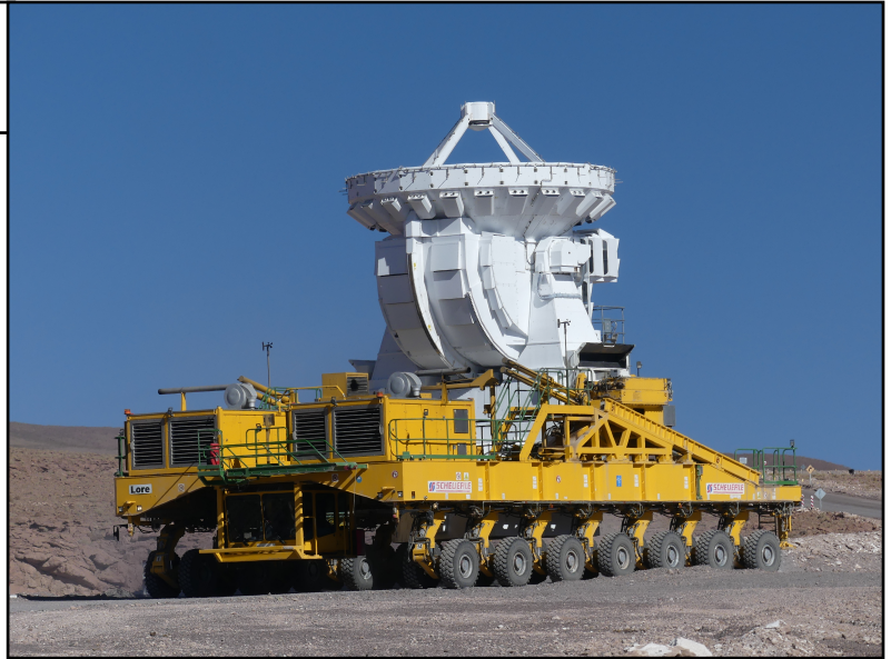
Figure 36: The ALMA transporter carrying one of the 7-m Array antennas to the OSF for servicing. (Credit G. Schieven)
