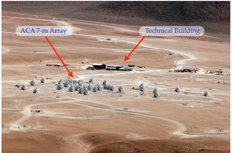
Figure 6: An aerial view of ALMA in a relatively compact configuration. The maximum distance between the 12-m Array antennas in the most compact configuration is less than 200 m, and are as close together as 15 m. Indicated also are the AOS Technical Building, and the ACA 7-m Array (Credit: C. Padilla/ALMA (ESO/NAOJ/NRAO))
