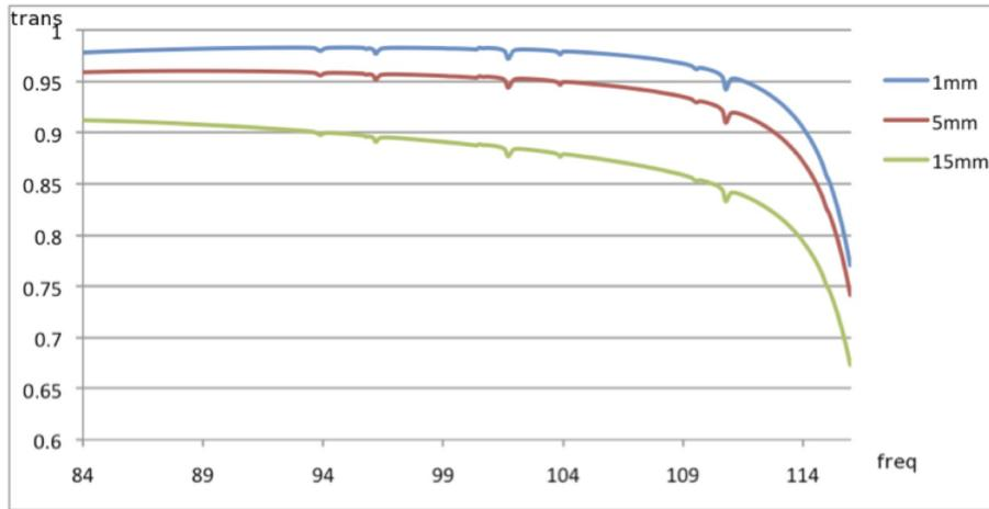
Figure 4.6: Band 3 zenith transmission for 1, 5 and 15 mm of PWV. Frequency is in GHz.
