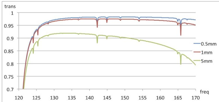
Figure 4.10: Band 4 zenith transmission for 0.5, 1 and 5 mm of PWV. Frequency is in GHz.
