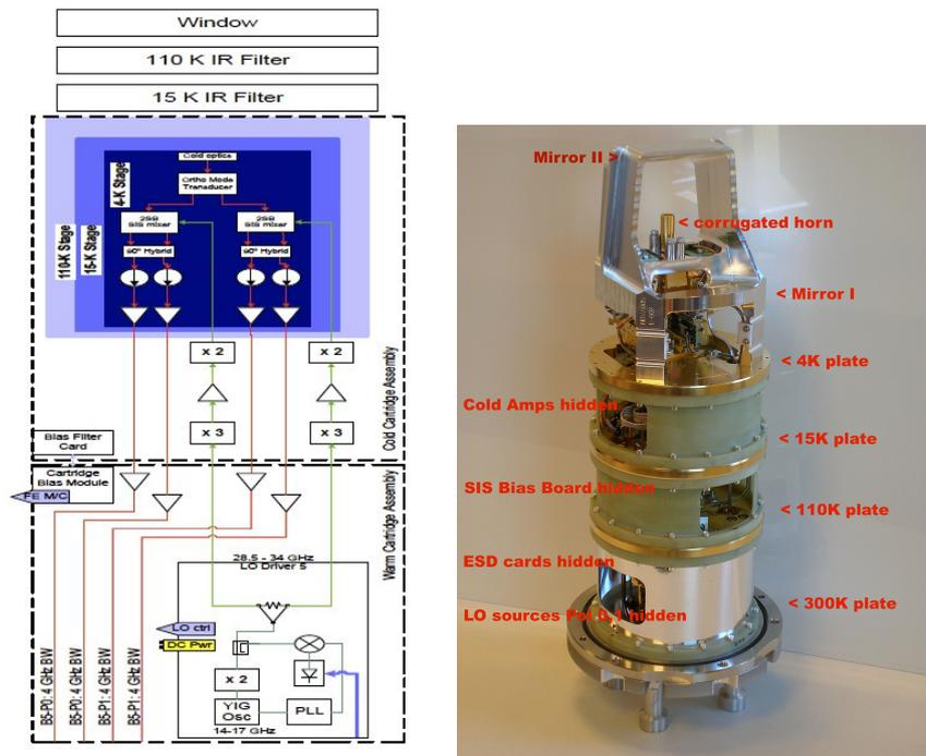
Figure 4.13: Block diagram of the Band 5 receiver (left) including CCA (upper) and WCA (lower). Right image shows a Band 5 CCA. Note the single feedhorn which feeds the OMT, splitting the two polarization signals for the 2SB SIS mixers. The active multiplier (x3, a power amplifier, then x2) is mounted between the 300 K and 110 K stage.
