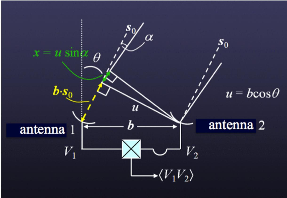
Figure 3.4: An ideal 1-D two-antenna interferometer consisting of two antennas, 1 and 2, separated by physical distance (i.e., a baseline)  $b$ . The antennas are both pointed towards a sky location given by  $s_o$ , which is at an angle  $\theta$  from the meridian. The projected distance between the two antennas in that direction is thus  $u = b \cos \theta$ . The two antennas are connected to a correlator where the voltages detected from each are combined.
