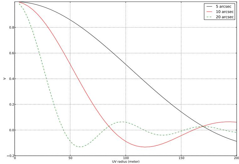
Figure 7.13: Annularly averaged amplitudes of the expected visibilities of three model uniform disks (annular averages) at 100 GHz as a function of  $uv$ -distance.
