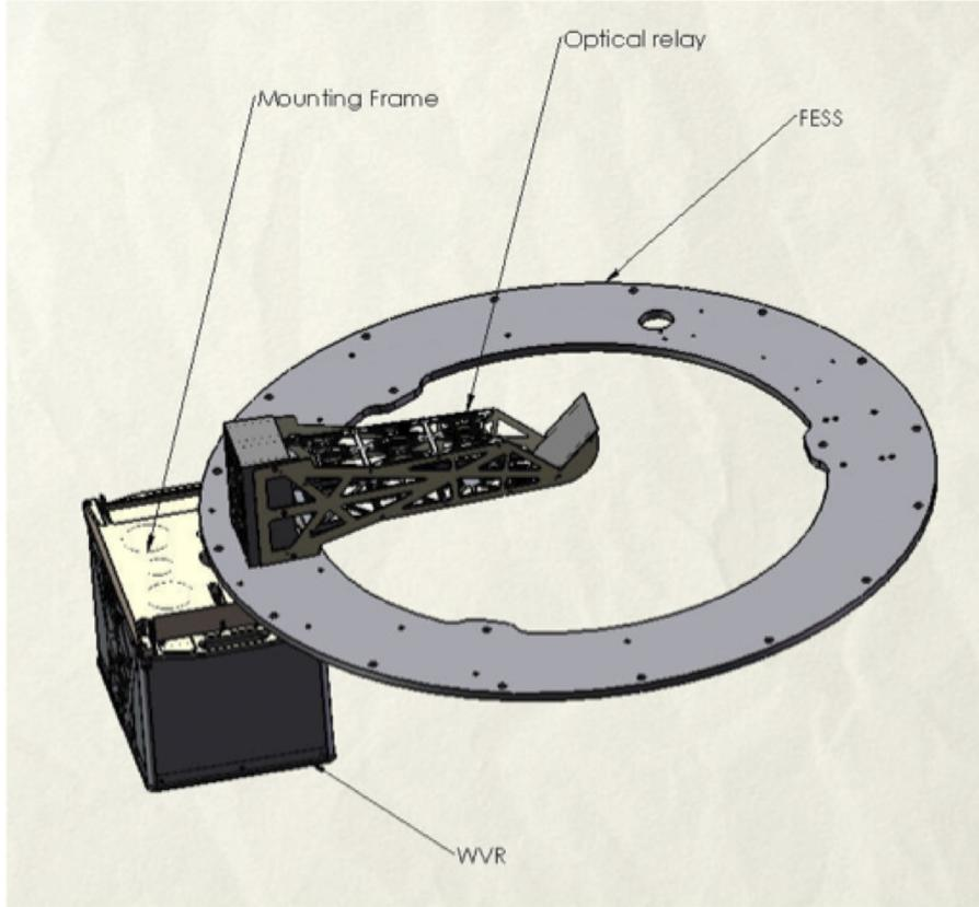
Figure A.10: Offset optics used to collect the sky emission along the optical axis of the antenna into the WVR.
