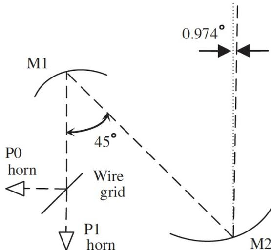
Figure 4.32: Schematic of ALMA Band 10 optics. ALMA Band 10 optics are composed of two elliptical mirrors, M1 and M2, a wire grid and two corrugated horns. The wire grid is used to separate the two linear polarizations, P0 and P1, and it is located after the two elliptical mirrors to minimize the number of optical components required.
