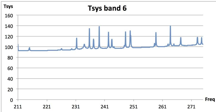
Figure 4.19: Typical  $T_{\text{sys}}$  at zenith for Band 6 with 1.262 mm PWV, based on measured values of the receiver temperatures.  $T_{\text{sys}}$  was computed using only the receiver temperature values adopted in the OT and the atmospheric contribution. No spill-over or background terms have been included. Temperature is given in Kelvin.
