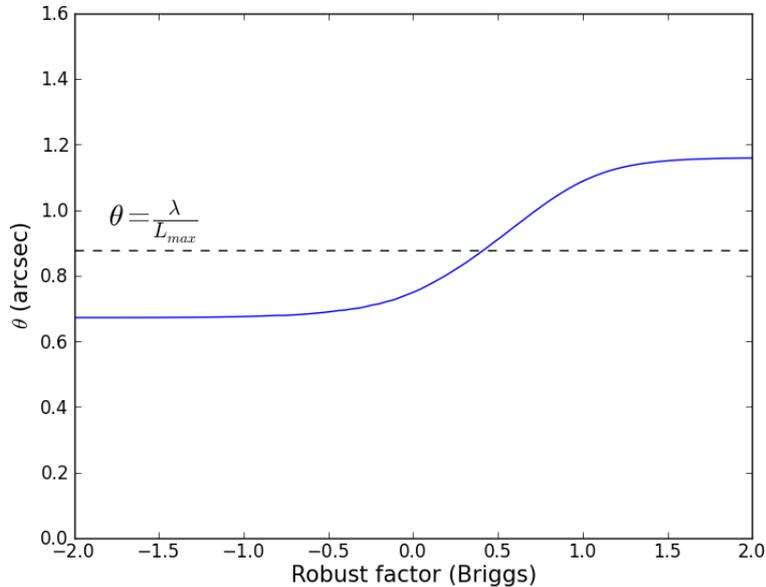
Figure 7.6: Angular resolution achieved using different values of the CASA *robust* parameter for a 1-hour observation at 100 GHz and a declination of -23 deg in the C43-4 configuration. Note that *robust* = -2 is close to uniform weighting and *robust* = 2 is close to natural weighting. The dotted line corresponds to  $\frac{\lambda}{L_{max}}$ .
