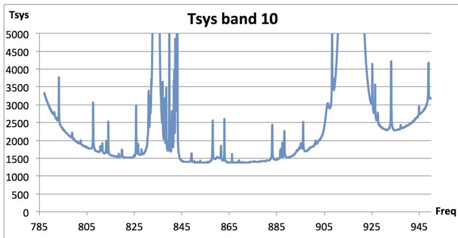
Figure 4.35: Typical  $T_{\text{sys}}$  at zenith for Band 10 with PWV = 0.472 mm.  $T_{\text{sys}}$  was computed using only the receiver temperature values adopted in the OT and the atmospheric contribution. No spill-over or background terms have been included. Temperature is given in Kelvin.
