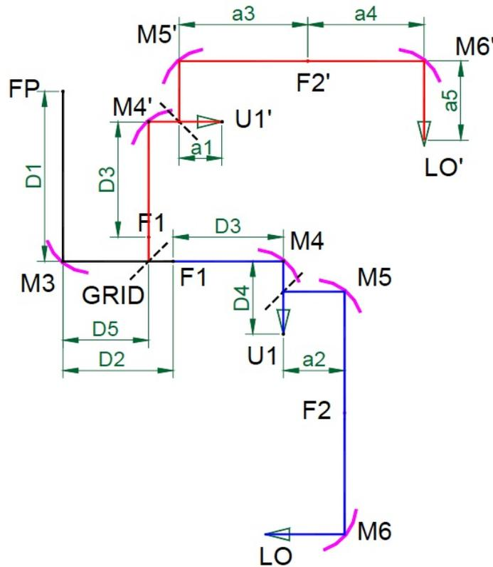
Figure 4.28: Basic Band 9 optics layout. The signal path is symmetrical for the vertical polarization (P0) and the horizontal polarization (P1). For P1 the path is as follows: a telescope focal point followed by mirror M3, grid, mirror M4, a beam splitter for LO insertion and finally the mixer horn U1. For P0 the signal follows from FP to the same mirror M3 and then, reflected by the grid, comes to mirror M4, a beam splitter, and mixer horn U1.
