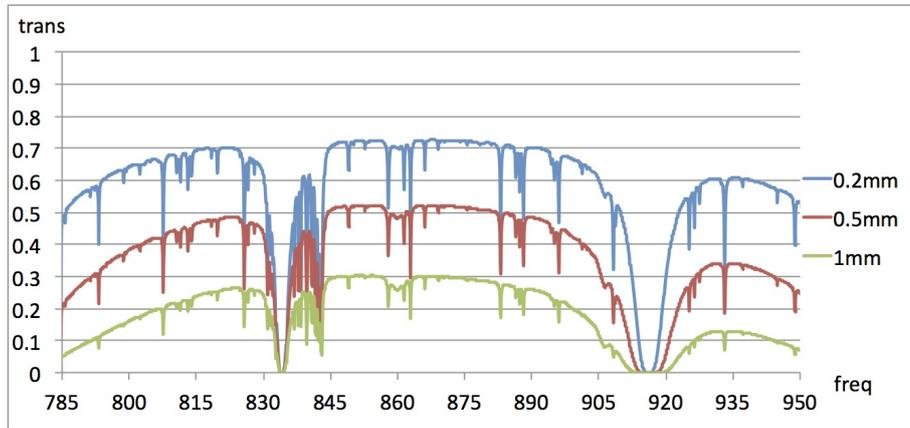
Figure 4.34: Band 10 zenith transmission for PWV = 0.2, 0.5 and 1 mm. Frequency is in GHz.
