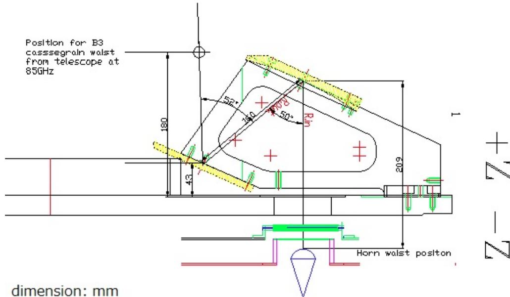
Figure 4.4: Input optics for Band 3, showing the warm pickoff mirrors. The location of the antenna beam from the secondary mirror is shown by the solid line, and the Cassegrain focus is shown by the small circle to the upper right.
