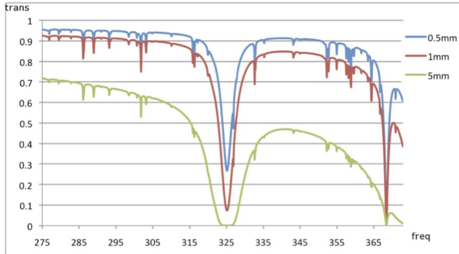
Figure 4.22: Band 7 atmospheric zenith transmission for PWV=0.5, 1.0 and 5.0 mm. Frequency is in GHz. The deep atmospheric absorption at 325 GHz is due to water, and the narrower feature at 369 GHz is due to oxygen.
