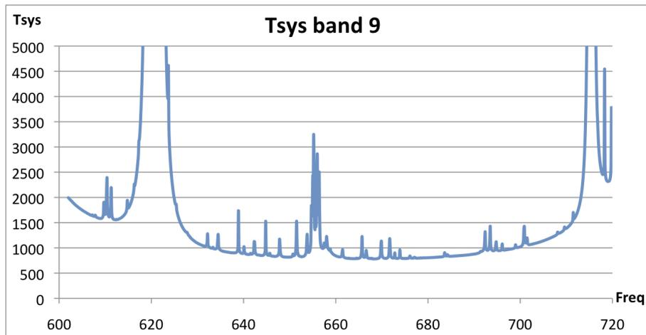
Figure 4.31: Typical  $T_{\text{sys}}$  at zenith for Band 9 with PWV = 0.472 mm.  $T_{\text{sys}}$  was computed using only the receiver temperature values adopted in the OT and the atmospheric contribution. No spill-over or background terms have been included. Temperature is given in Kelvin.
