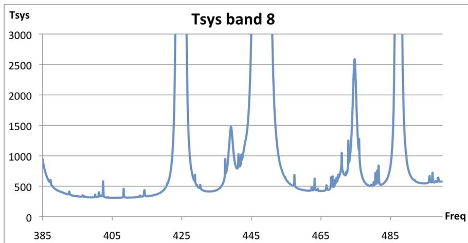
Figure 4.27: Typical  $T_{\text{sys}}$  at zenith for Band 8 with PWV=0.472 mm.  $T_{\text{sys}}$  was computed using only the receiver temperature values adopted in the OT and the atmospheric contribution. No spill-over or background terms have been included. Temperature is given in Kelvin.
