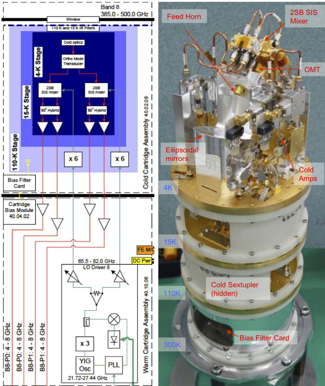
Figure 4.25: Block diagram of the Band 8 receiver (left) including CCA (upper) and WCA (lower). Right image shows a Band 8 CCA. Note the single feedhorn which feeds the OMT, splitting the two polarization signals for the 2SB SIS mixers. The Band 8 cartridges were constructed at the Advanced Technology Center (ATC).
