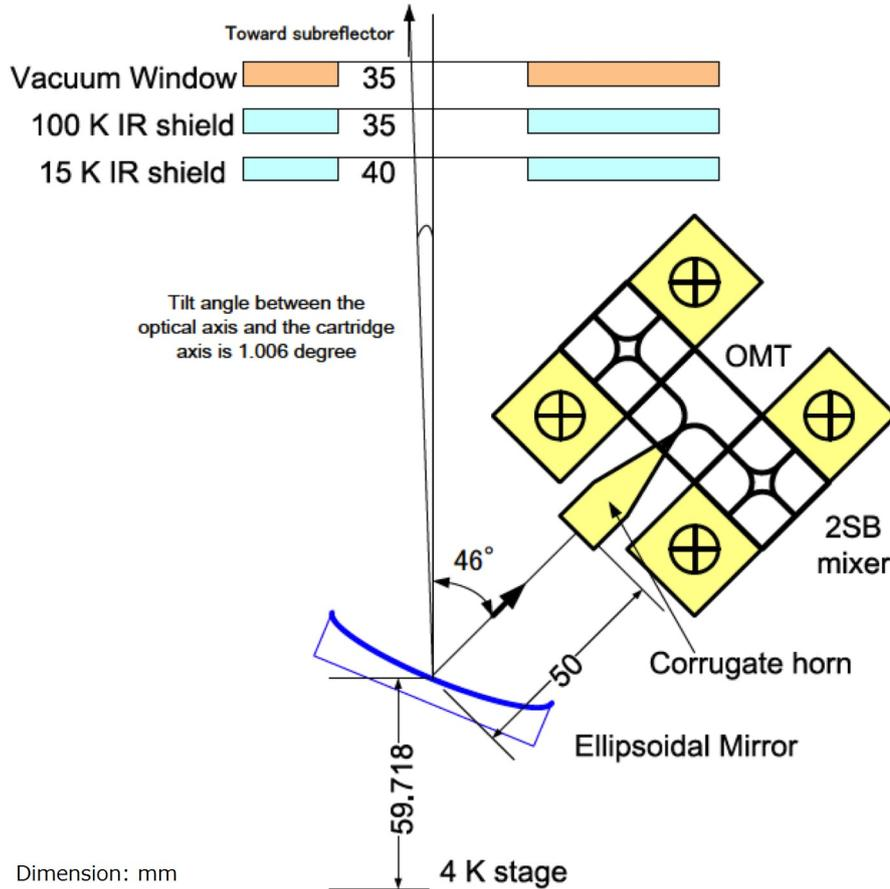
Figure 4.24: Optical layout of the Band 8 receiver.
