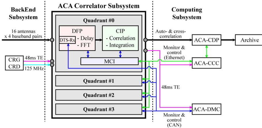
Figure 5.5: Overview diagram of the ACA Correlator. The signals from the BackEnd Subsystem are processed in the DFP and CIP modules and output to the Computing Subsystem (see text and Figure 5.3 for details of these). The modules are controlled by the Monitor and Control Interface (MCI), which communicates with the correlator control computer (ACA-CCC). The DTS-Rx is connected with the monitor and control computer (ACA-DMC) for the monitor and control compatibility with the 64-input Correlator.
