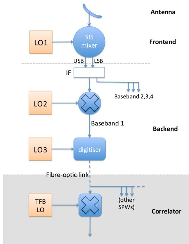
Figure 6.1: Summary block diagram of ALMA signal path and LO system for one spectral window, one baseband, one polarisation. The Backend IF system is located in each antenna, and the digitised signal for each baseband/polarisation is fed to the correlator in the central technical building through buried optical fibers. See Appendix B for a more detailed description of the components and the other tasks that the LO systems perform.
