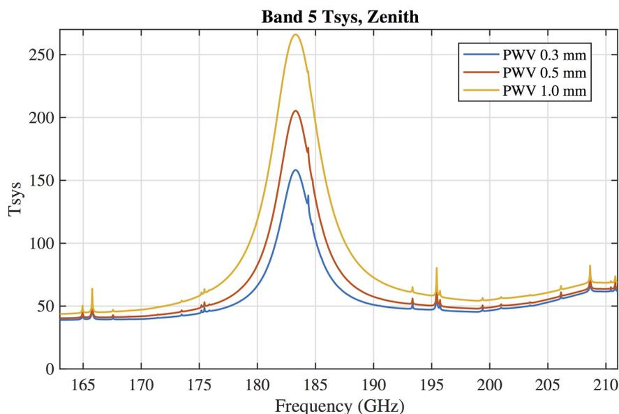
Figure 4.15: Typical system temperature ( $T_{sys}$ ) at zenith for Band 5 for three typical PWV values. ( $T_{sys}$  was computed using only the receiver temperature values adopted in the OT and the atmospheric contribution. No spill-over or background terms have been included. Temperature is given in Kelvin.)
