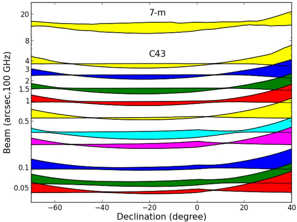
Figure 7.9: Cycle 5 angular resolutions as a function of source declination. Each color shows, for a particular configuration, the range of the major and minor axes of the synthesized beams expected from a 2-hour observation at 100 GHz and at transit. 12-m Array configurations are arranged with C43-1 at the top and C43-10 at the bottom.
