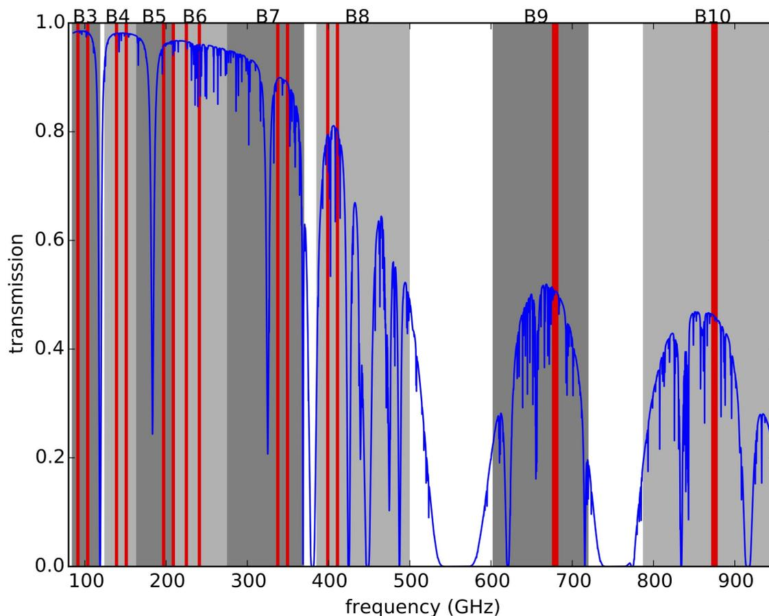
Figure 6.2: ALMA bands available in Cycle 5 (Bands 3 - 10), showing the frequency of the standard continuum settings as red shading. This gives the coverage of both USB and LSB, except for Bands 9 and 10, which have 8 GHz of bandwidth using the USB only. The available frequency coverage of each band is shown by the grey shading, and atmospheric transmission for 0.6 mm of PWV is given by the blue line.
