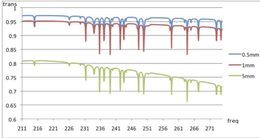
Figure 4.18: Band 6 zenith transmission for PWV=0.5, 1 and 5 mm. Frequency is in GHz. Most of the narrow absorption lines are from ozone.
