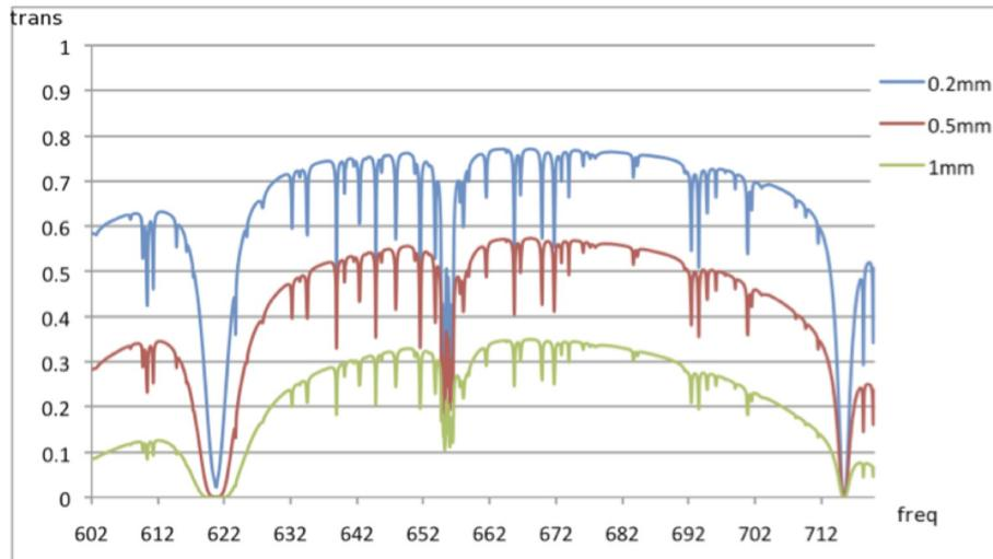
Figure 4.30: Band 9 zenith transmission for PWV = 0.2, 0.5 and 1 mm. Frequency is in GHz.
