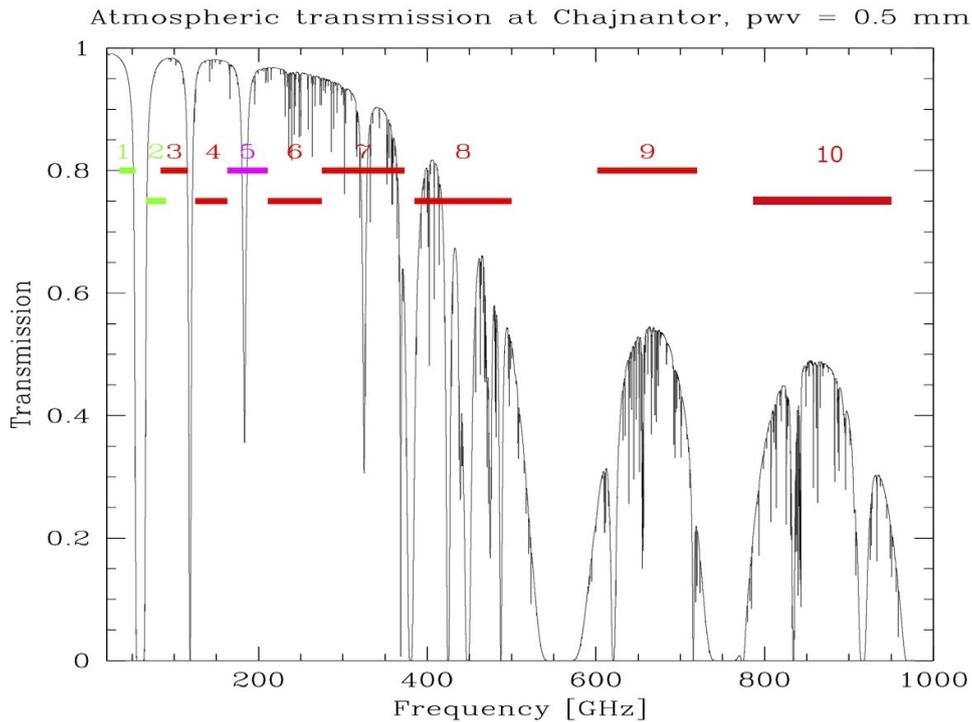
Figure 4.1: The ten ALMA receiver bands. Receiver bands for Cycle 5 are shown in red or purple superimposed on a zenith atmospheric transparency plot at the Array Operation Site (AOS) for 0.5 mm of Precipitable Water Vapor (PWV). Band 5 (shown in purple) is newly available in Cycle 5.
