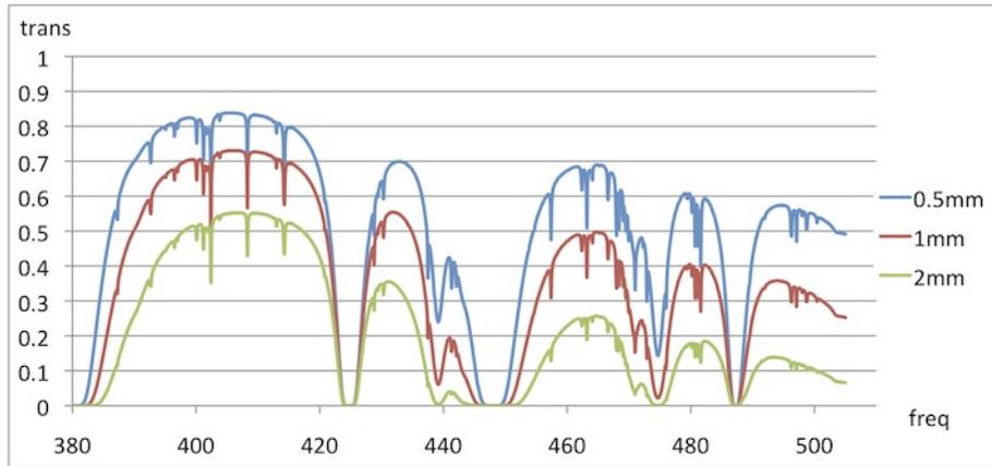
Figure 4.26: Band 8 atmospheric zenith transmission for PWV=0.5, 1.0 and 2.0 mm. Frequency is in GHz. The atmosphere in the Band 8 frequency range has some deep absorption by water and oxygen.
