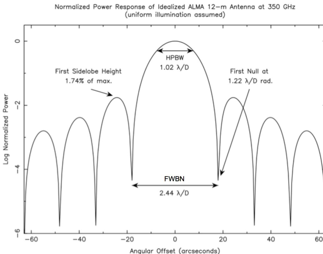
Figure 3.3: Normalized 1-D antenna power response for a 12 m antenna uniformly illuminated at 300 GHz. The power is in log units to emphasize the sidelobes. The HPBW of the primary beam is  $\sim 1.02 \lambda/D$  and the FWBN is  $\sim 2.44 \lambda/D$ . The angle of the first null, i.e., the resolution, is  $0.5 \times \text{FWBN} = \sim 1.22 \lambda/D$ . Note that the HPBW measured from actual 12 m ALMA antennas is  $\sim 1.13 \lambda/D$  because the illumination is not uniform.
