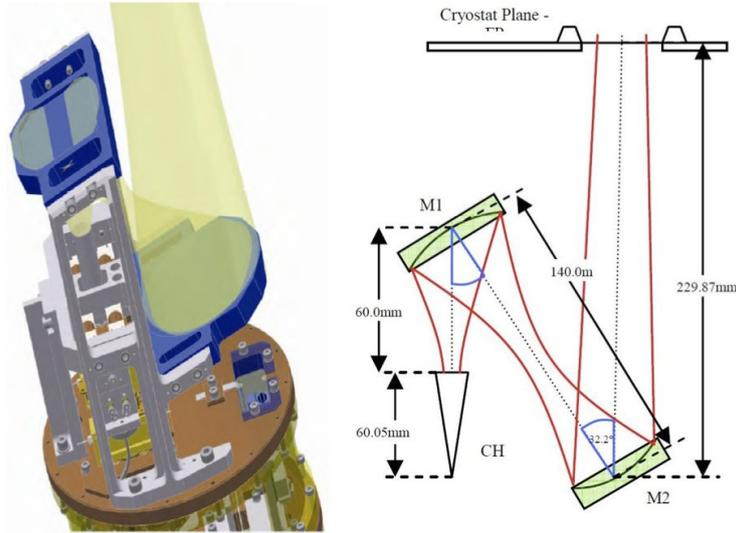
Figure 4.12: Optical layout of the Band 5. Placing the mixer assembly along the side of M 1 and streamlined layout of the IF system are the key to fulfil the requirements on  $5w_o$  optical beam clearance.
