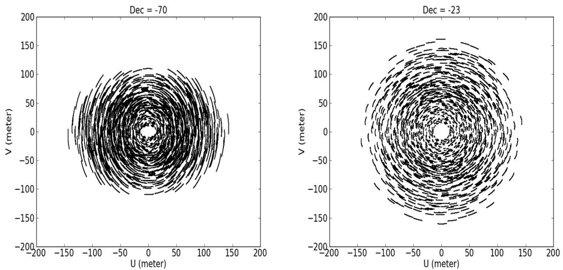
Figure 7.8:  $uv$ -plane coverage for configuration C43-1 with a 1-hour observation of a transiting source at a declination of either  $-70^\circ$  (left) or  $-23^\circ$  (right). For the source with a declination of  $-70^\circ$ , the shadowing fraction represents 25.7% of the total.
