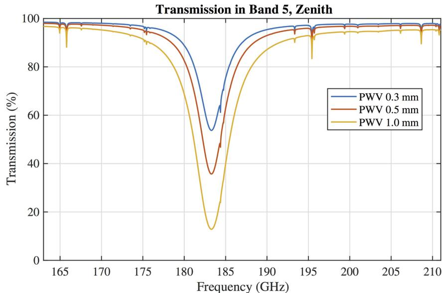
Figure 4.14: Band 5 zenith transmission for 0.5, 1 and 5 mm of PWV. Frequency is in GHz.
