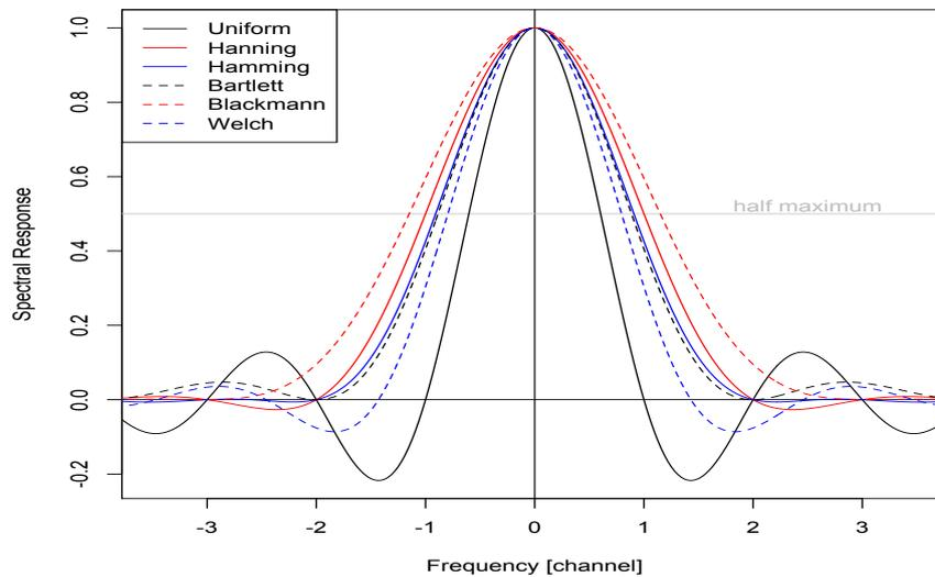
Figure 5.7: Spectral resolution functions corresponding to various weighting functions
