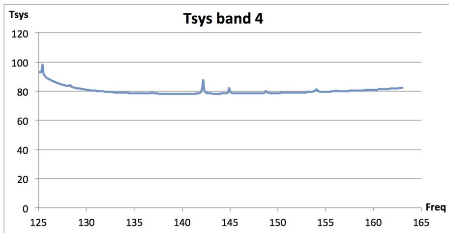
Figure 4.11: System temperature ( $T_{\text{sys}}$ ) at zenith for Band 4 with 1.262 mm of PWV.  $T_{\text{sys}}$  was computed using only the receiver temperature values adopted in the OT and the atmospheric contribution. No spill-over or background terms have been included. Temperature is given in Kelvin.
