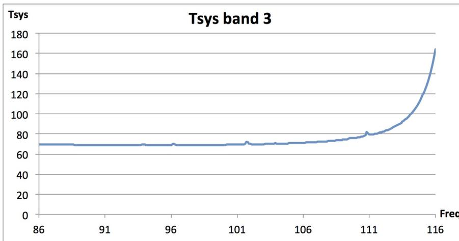
Figure 4.7: Typical system temperature ( $T_{\text{sys}}$ ) at zenith for Band 3 with 1.262 mm of PWV.  $T_{\text{sys}}$  was computed using only the receiver temperature values adopted in the OT and the atmospheric contribution. No spill-over or background terms have been included. Temperature is given in Kelvin.
