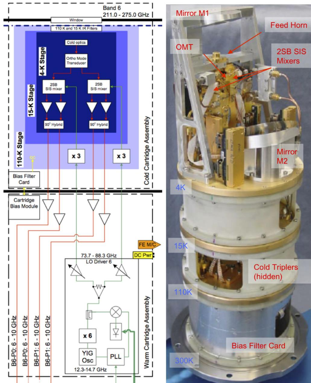
Figure 4.17: Band 6 receiver block diagram, and (right) image of cartridge. Note the OMT used to split the polarizations feeding the two 2SB mixers. The LO around 80 GHz requires an extra  $\times 3$  multiplier inside the cryostat. The Band 6 cartridges were built at NRAO, Charlottesville. Note that the IF output range is actually 5-10 GHz; the range shown is the one recommended for continuum observations (see text).
