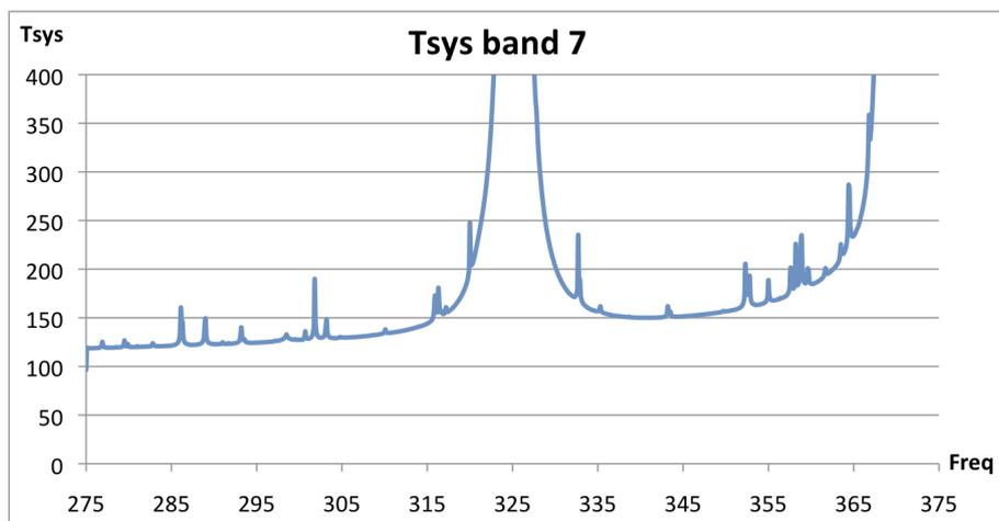
Figure 4.23: Typical  $T_{\text{sys}}$  at zenith for Band 7 with PWV=0.913 mm.  $T_{\text{sys}}$  was computed using only the receiver temperature values adopted in the OT and the atmospheric contribution. No spill-over or background terms have been included. Temperature is given in Kelvin.
