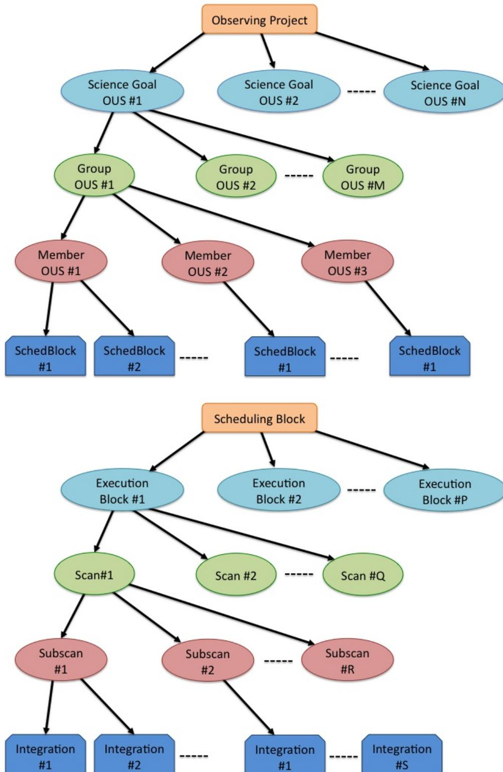
Figure 8.1: Block diagram of an Observing Project from the point of view of the observation preparation (top) and internal hierarchical structure of the SB in actual executions (bottom). All projects have the same ObsUnitSet (OUS) levels, the Science Goal OUS level, the Group OUS level and the Member OUS level. Scheduling blocks are attached to the Member OUS. Each time a Scheduling Block is executed, Control creates a new ExecBlock structure (see text).
