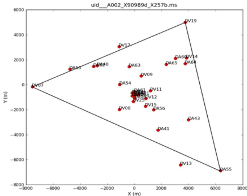
Figure 8: LBC array as of mid-October during the middle of the imaging and SV phase of the campaign. Note this includes the moves of antennas DA55 and DV07 to achieve a baseline >15 km.
