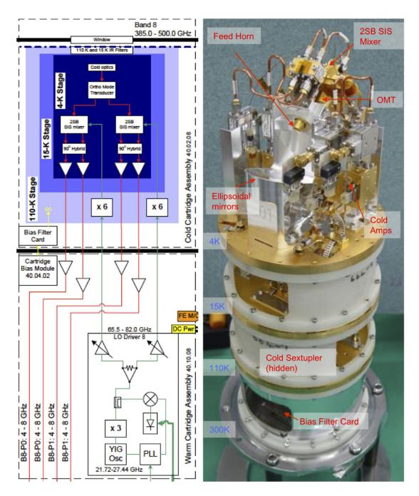
Figure 4.29: Block diagram of the Band 8 receiver (left) including CCA (upper) and WCA (lower). Right image shows a Band 8 CCA. Note the single feedhorn which feeds the OMT, splitting the two polarization signals for the 2SB SIS mixers. The Band 8 cartridges were constructed in Japan at the NAOJ Advanced Technology Center (ATC) in Mitaka, Japan.
