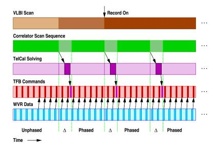
Figure 8.8: VLBI Scans in the Phasing System. Each VLBI scan is partitioned into "subscans" for correlation and "slow" timescale processing (of order seconds) in TelCal. WVR adjustments are made in the CDP on a "fast" timescale (every second). See text for full discussion and explanation.
