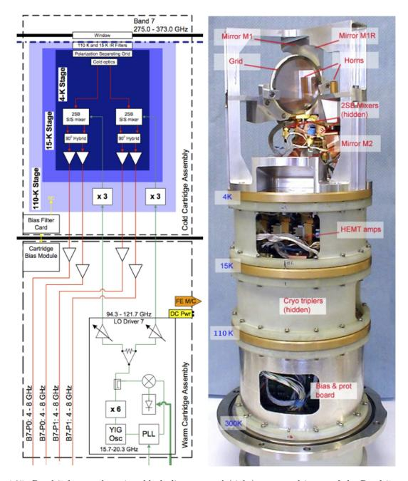
Figure 4.25: Band 7 front-end receiver block diagram, and (right) annotated image of the Band 7 cartridge. Note the polarization-splitting grid and LO injection in the cold optics above the mixers. The Band 7 cartridges were built in France at the Institut de Radio Astronomie Millimétrique (IRAM) in Grenoble, France.
