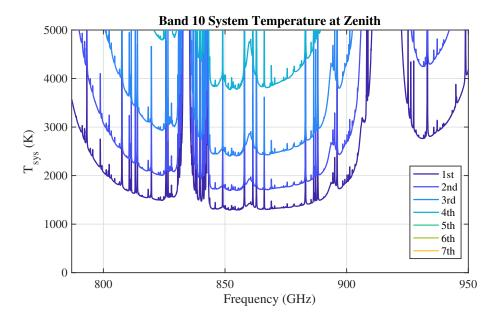
Figure 4.39: Typical  $T_{\rm sys}$  at zenith with Band 10 for the first seven octiles of observing conditions at ALMA. Note that the values for  $T_{\rm sys}$  in the worst octiles, which should never be used for high-frequency observations, are off scale in this plot.  $T_{\rm sys}$  was computed using only the receiver temperature values adopted in the ALMA OT and the atmospheric contribution. No spill-over or background terms have been included. Temperature is given in Kelvin.
