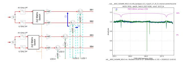
Figure C.2: (left) Possible route of interference from LO2-2 into LO2-1 or IF2-1 signals inside an IFP. (right) Bandpass spectrum affected by the LO2 leakage. The bandpass spectrum is produced by a cross-power spectrum normalized by a power spectrum (autocorrelation) where the leakage contaminates.
