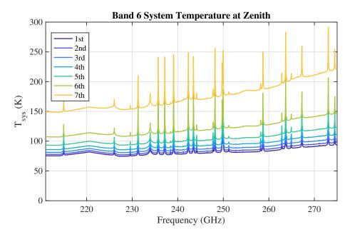
Figure 4.23: Typical system temperature  $(T_{\rm sys})$  at zenith for Band 6 for the first seven octiles of observing conditions at ALMA, based on measured values of the receiver temperatures.  $T_{\rm sys}$  was computed using only the receiver temperature values adopted in the ALMA OT and the atmospheric contribution. No spill-over or background terms have been included. Temperature is given in Kelvin.
