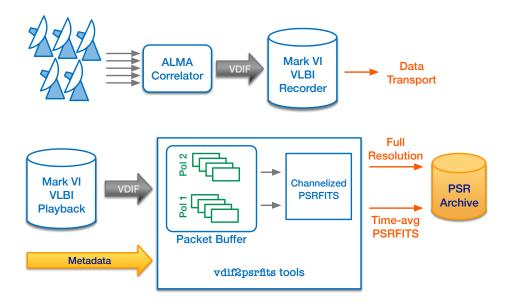
Figure 8.9: Diagram showing the data flow during a pulsar mode (PM) observation. Baseband data recorded at ALMA will be sent to MPIfR (Bonn, Germany) for playback and PRSFITS generation. Reproduced from Figure 2 of Liu et al. (2019).
