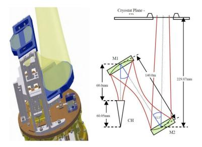
Figure 4.16: Optical layout of the Band 5. Placing the mixer assembly along the side of mirror M1 and the streamlined layout of the IF system are the key to fulfill the requirements on  $5w_{\rm o}$  optical beam clearance at the entrance to the cryostat.
