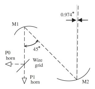
Figure 4.36: Schematic of ALMA Band 10 optics. ALMA Band 10 optics are composed of two elliptical mirrors, M1 and M2, a wire grid and two corrugated horns. The wire grid is used to separate the two linear polarizations, P0 and P1, and it is located after the two elliptical mirrors to minimize the number of optical components required.
