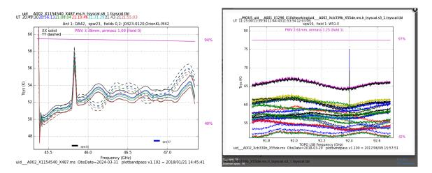
Figure C.1: (left) WVR LO leakage appeared at 45.825 GHz in the Tsys spectrum of Band 1. (right) RFI at 92.4 GHz emitted by APEX holography beacon.
