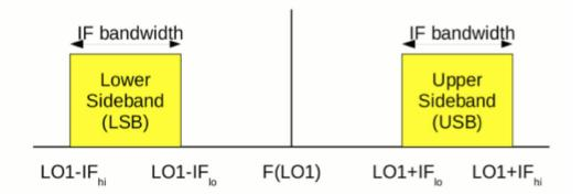
Figure 4.2: IF ranges for the two sidebands in a heterodyne receiver.
