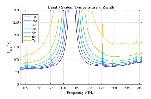
Figure 4.19: Typical system temperature  $(T_{\text{sys}})$  at zenith for Band 5 for the first seven octiles of observing conditions at ALMA.  $T_{\text{sys}}$  was computed using only the receiver temperature values adopted in the ALMA OT and the atmospheric contribution. No spill-over or background terms have been included. Temperature is given in Kelvin.
