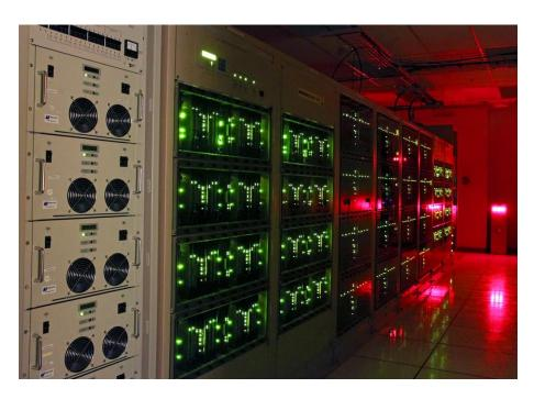
Figure 5.1: The ALMA 64-input Correlator. This view shows lights glowing on some of the racks of the correlator in the ALMA Array Operations Site Technical Building and shows one of four quadrants of the correlator. Credit: ALMA (ESO/NAOJ/NRAO), S. Argandoña
