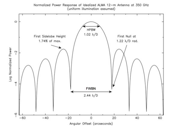
Figure 3.3: Normalized 1-dimensional (1-D) antenna power response for a 12-m antenna uniformly illuminated at 350 GHz. The power is in log units to emphasize the sidelobes. The HPBW of the primary beam is ~1.02  $\lambda/D$  and the FWBN is ~2.44  $\lambda/D$ . The angle of the first null, i.e., the resolution, is  $0.5 \times \text{FWBN} = ~1.22 \lambda/D$ . Note that the HPBW measured for actual ALMA 12-m and 7-m antennas is ~1.13  $\lambda/D$  because the illumination is not uniform.
