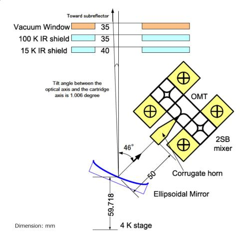
Figure 4.28: Optical layout of the Band 8 receiver.
