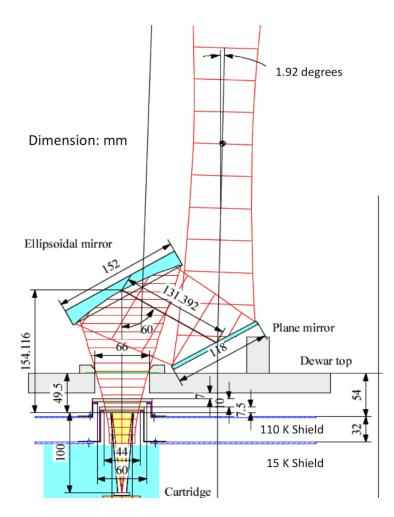
Figure 4.12: Optical layout of the Band 4 receiver. A beam width of 5 times the Gaussian beam size (w) is indicated in red.
