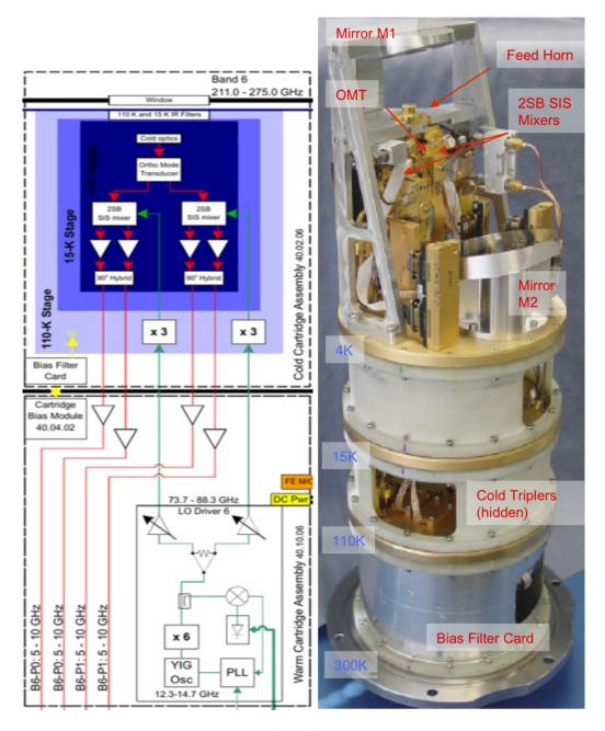
Figure 4.21: Band 6 receiver block diagram, and (right) image of cartridge. Note the OMT used to split the polarizations feeding the two 2SB mixers. The LO around 80 GHz requires an extra  $\times 3$  multiplier inside the cryostat. Note that the IF output range has been extended to cover 4.5–10 GHz; the range shown is the one recommended for continuum observations (see text). The Band 6 cartridges were built in the United States at the NRAO Technology Center in Charlottesville, Virginia.
