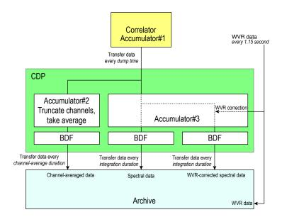
Figure 5.6: Basic data processing and accumulation/averaging steps between the correlator and archive. The CDP applies channel truncation, spectral averaging, and time averaging for the channel-averaged data. It also applies online WVR correction to produce the WVR-corrected spectral data. They are packed in Binary Data Format (BDF) and are archived together with the WVR data.
