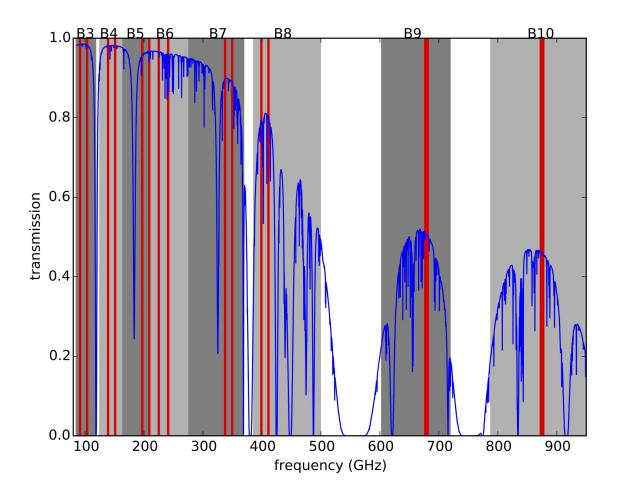
Figure 6.2: ALMA bands available in Cycle 12 (Bands 1, 3 - 10), showing the frequency of the standard continuum settings as red shading. This gives the coverage of both USB and LSB, except for Bands 9 and 10, which have 8 GHz of bandwidth using the USB only. The available frequency coverage of each band is shown by the grey shading, and atmospheric transmission for 0.6 mm of PWV is given by the blue line.
