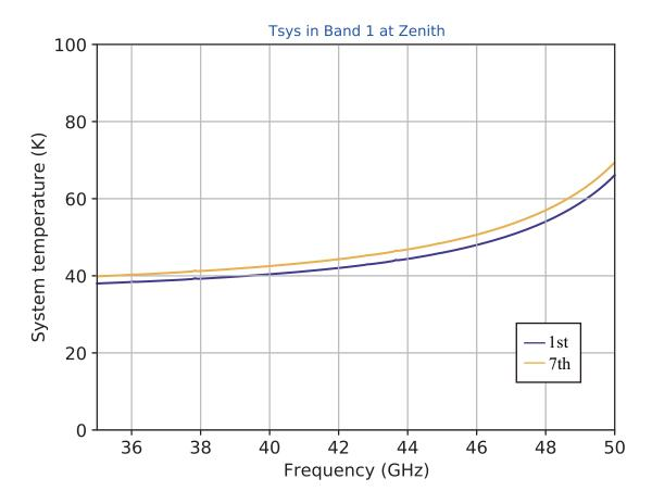
Figure 4.7: Band 1 zenith Tsys for the first and seventh octiles of observing conditions at ALMA. Receiver temperature  $(T_{\rm RX})$  is assumed to be 28K. Note that the full frequency range of Band 1 can be covered in two LO1 frequency settings.
