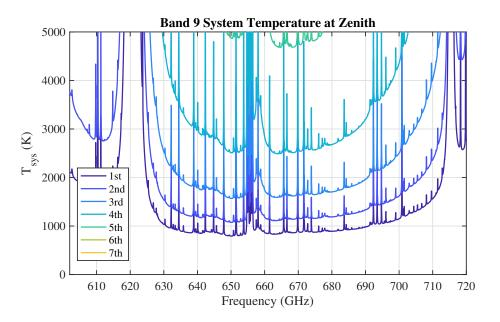
Figure 4.35: Typical  $T_{\rm sys}$  at zenith for Band 9 for the first seven octiles of observing conditions at ALMA. Note that the values for  $T_{\rm sys}$  in the worst octiles, which should never be used for high-frequency observations, are off scale in this plot.  $T_{\rm sys}$  was computed using only the receiver temperature values adopted in the ALMA OT and the atmospheric contribution. No spill-over or background terms have been included. Temperature is given in Kelvin.
