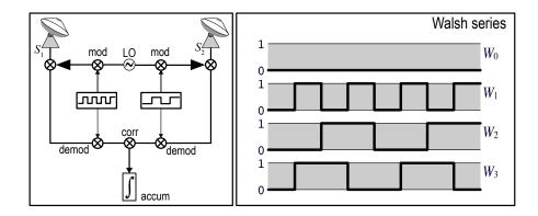
Figure 5.7: Schematic diagram of phase switching. The LO1 signal phase is modulated with the Walsh series pattern and demodulated in the DTS before cross-correlation. The Walsh function series are employed to generate switching patterns that are orthogonal to each other.
