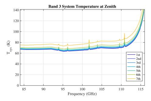
Figure 4.11: Typical system temperature  $(T_{\rm sys})$  at zenith for Band 3 for the first seven octiles of observing conditions at ALMA.  $T_{\rm sys}$  was computed using only the receiver temperature values adopted in the ALMA OT and the atmospheric contribution. No spill-over or background terms have been included. Temperature is given in Kelvin.
