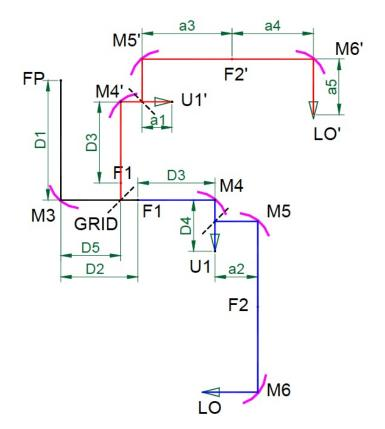
Figure 4.32: Basic Band 9 optics layout. The signal path is symmetrical for the vertical polarization (P0) and the horizontal polarization (P1). For P1 the path is as follows: the telescope focal point (FP) is followed by mirror M3, wire grid polarization splitter, mirror M4, a beam splitter for LO insertion, and finally the mixer horn U1. For P0 the signal follows from FP to the same mirror M3 and then, reflected by the grid, comes to mirror M4, a beam splitter, and mixer horn U1'.
