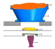
Figure 4.5: Cross-section of the ALMA Band 1 optics installed in the ALMA cryostat (Gonzalez et al. 2017). The lens (5) is placed on top of a lens holder (4) which provides the appropriate tilt and distance to the feed horn. The lens acts as cryostat window and holds vacuum. The incoming radiation must go through two IR filters placed on support rims on the 110K shield (3) and the 15K shield (2) before finally reaching the Band 1 corrugated horn (1).
