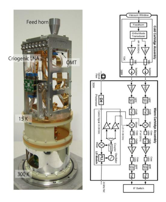
Figure 4.4: Left figure shows the Band 1 receiver cartridge (Courtesy: Teddy Huang (ASIAA)). Right figure shows the block diagram of the Band 1 receiver including CCA (upper) and WCA (lower) (Huang et al. 2016).
