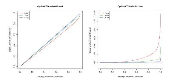
Figure 5.8: Van Vleck relationship of 2-, 3-, and 4-bit quantizations at the optimal signal power level and threshold voltages. (Left): Correlation coefficient of digitized signals as a function of analog correlation coefficients,  $\rho$ . (Right): Departures of the Van Vleck relationship from linear relation using the single factors of  $\eta_4 = 0.881$ ,  $\eta_8 = 0.963$ , and  $\eta_{16} = 0.988$  for 2-, 3-, and 4-bit quantizations, respectively.
