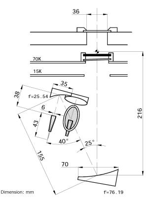
Figure 4.24: Band 7 cold optics arrangement, showing the off-axis ellipsoidal mirrors and the polarization splitter wire grid.
