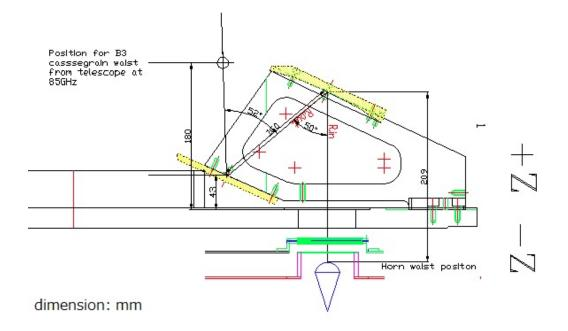
Figure 4.8: Input optics for Band 3, showing the warm pickoff mirrors. The location of the center of the antenna beam from the secondary mirror is shown by the vertical solid line, and the Cassegrain focus is shown by the small circle to the upper left.
