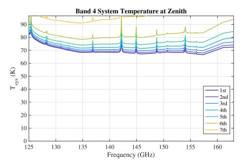
Figure 4.15: System temperature  $(T_{\text{sys}})$  at zenith for Band 4 for the first seven octiles of observing conditions at ALMA.  $T_{\text{sys}}$  was computed using only the receiver temperature values adopted in the ALMA OT and the atmospheric contribution. No spill-over or background terms have been included. Temperature is given in Kelvin.
