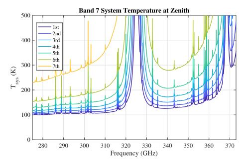
Figure 4.27: Typical  $T_{\rm sys}$  at zenith for Band 7 for the first seven octiles of observing conditions at ALMA.  $T_{\rm sys}$  was computed using only the receiver temperature values adopted in the ALMA OT and the atmospheric contribution. No spill-over or background terms have been included. Temperature is given in Kelvin.
