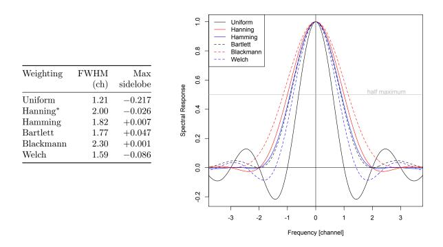
Figure 5.5: (left table) Spectral resolutions (FWHM) and the maximum sidelobe levels for weighting functions. ALMA employs the Hanning window in default. (right figure) Spectral resolution functions corresponding to various weighting functions
