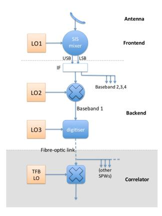
Figure 6.1: Summary block diagram of ALMA signal path and LO system for one spw, one baseband, one polarization. The Back-end IF system is located in each antenna, and the digitized signal for each baseband/polarization is fed to the correlator in the central technical building through buried optical fibers. See Appendix B for a more detailed description of the components and the other tasks that the LO systems perform.
